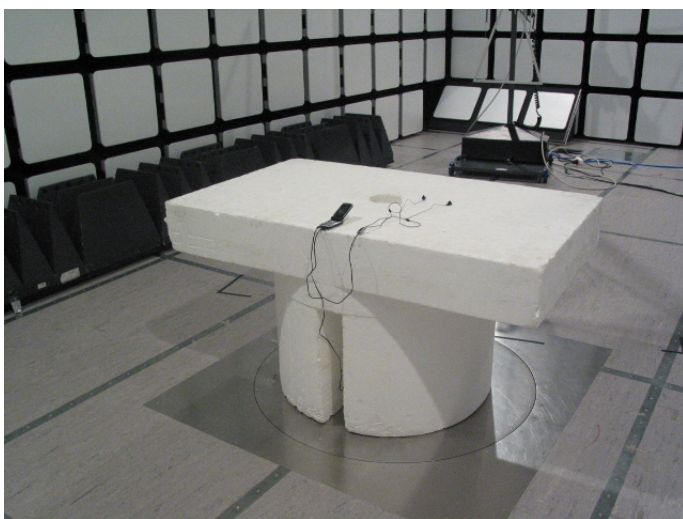
Picture 2 Radiated emission measurement WLAN TX
