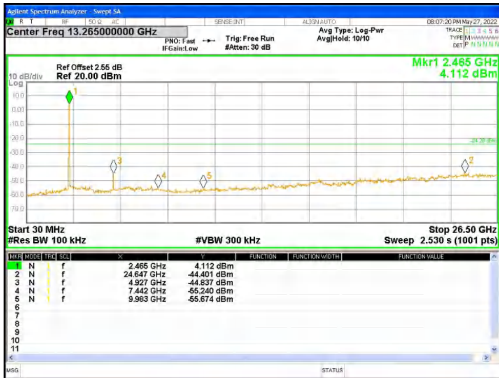
Tx. Spurious NVNT g 2412MHz Ant1 Ref
