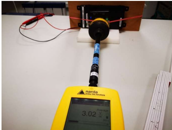
Photograph 5: Measurements in the shielded room, 7.3 cm distance between measurement probe and EUT, Position 5, E-Field, 90% charging level
