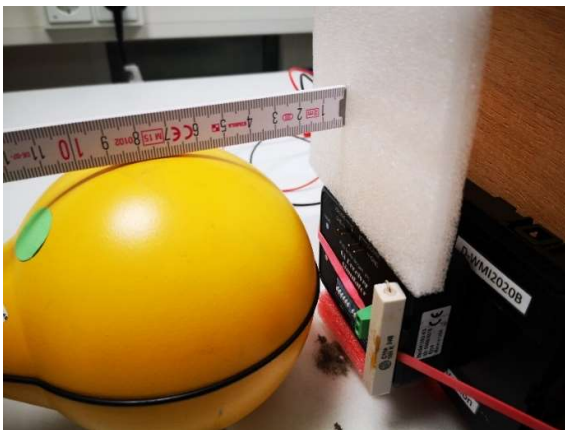
Photograph 29: Measurements in the shielded room, 7.3 cm distance between measurement probe and EUT, Position 5, H-Field, 50% charging level
