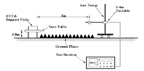
The radiated emission Below 1GHz tests were performed in the 3 meters chamber test site A, above 1GHz tests were performed in the 3 meters chamber test site B, using the setup accordance with the ANSI C63.4-2014. The specification used was the FCC Part 15.109 Class B limits.
