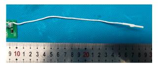
Antenna transmission frequency: 433.92MHz
