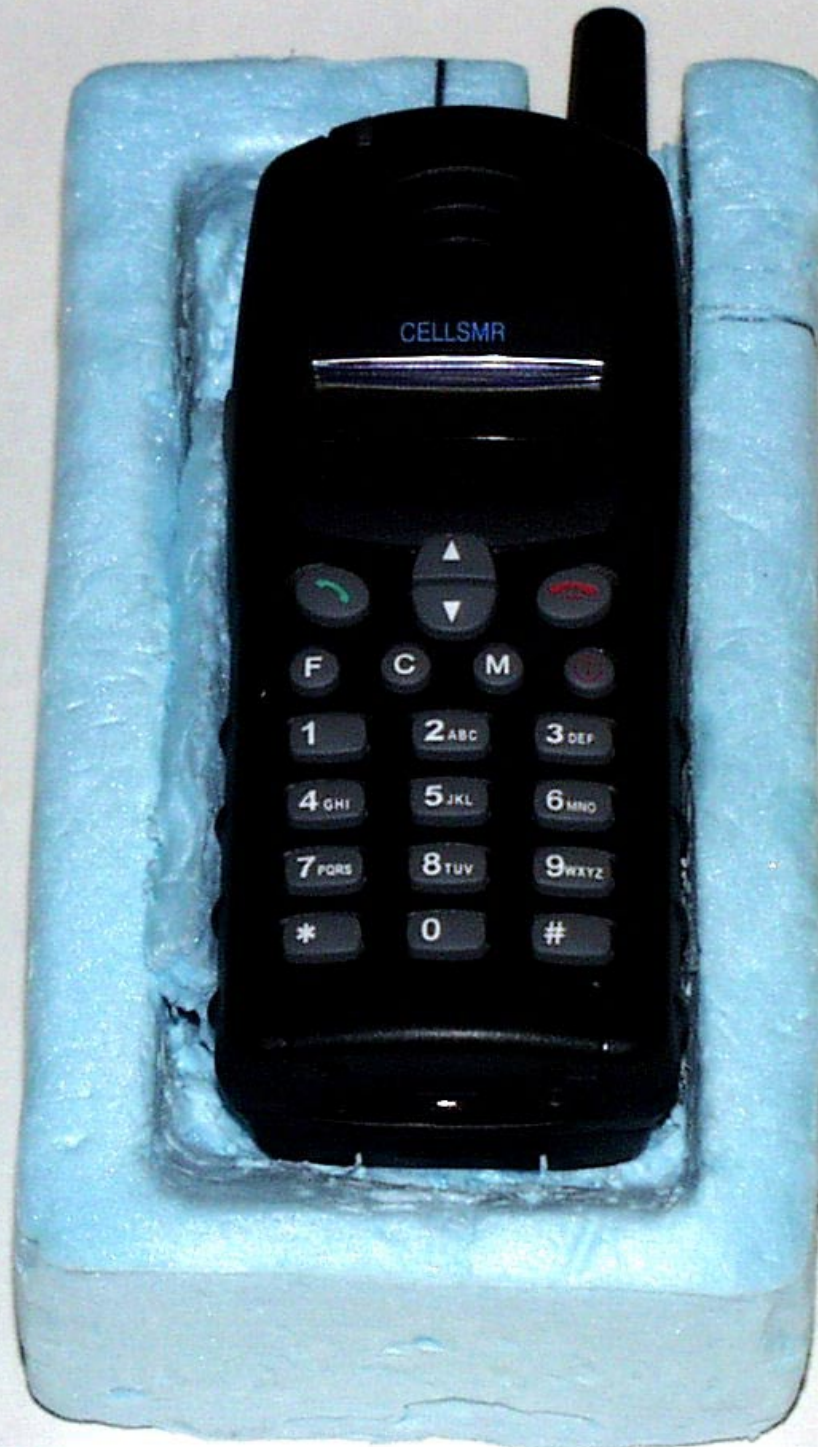
Fig.A Front view of the TECOM Model T-2000A in a Styrofoam holder for SAR testing. Note that the antenna is angled backwards.
