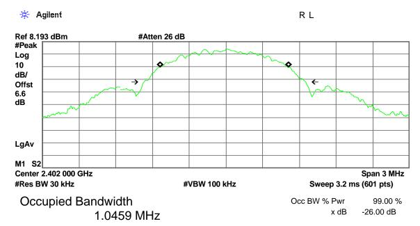
Transmit Freq Error -13.816 kHz x dB Bandwidth 1.327 MHz
