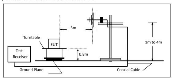
(c) For radiated emissions above 1000MHz
