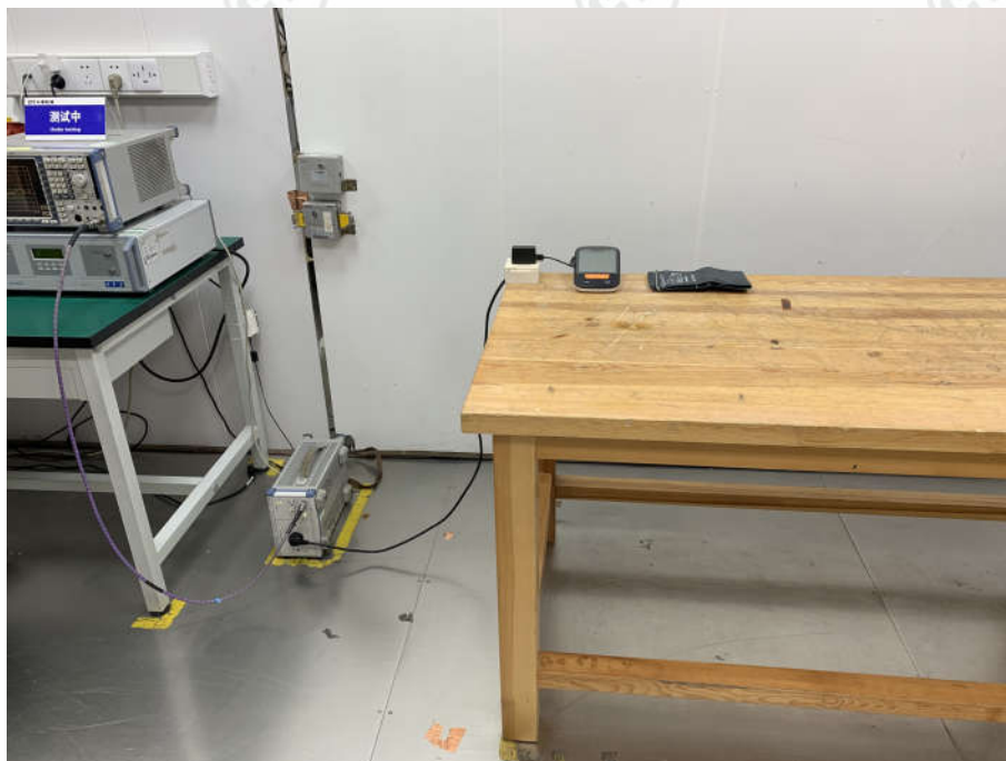
Conducted Emissions Test Setup
