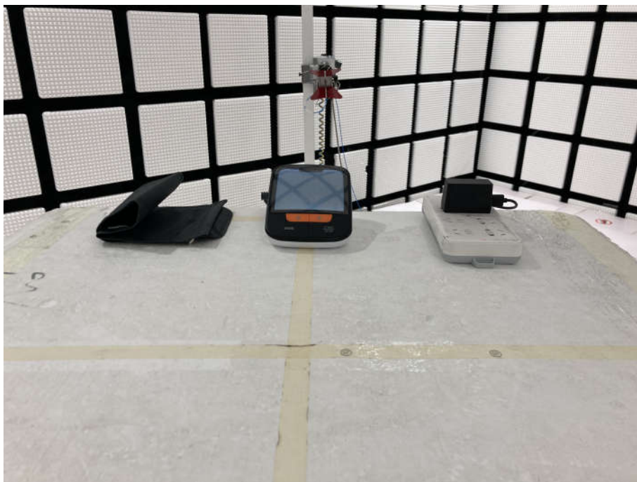
Radiated spurious emission Test Setup-2(Above 1GHz)
