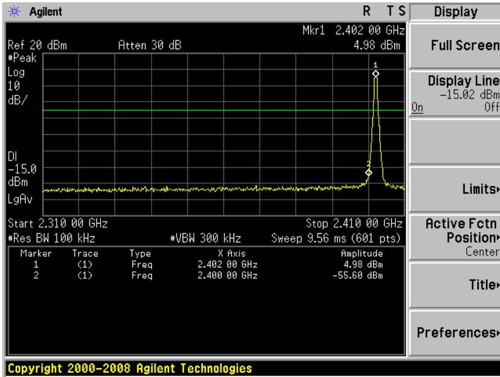
GFSK mode: Band Edge-High Channel
