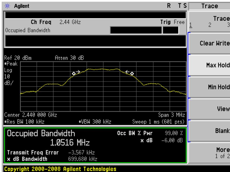
6dB Bandwidth plot on channel 39
