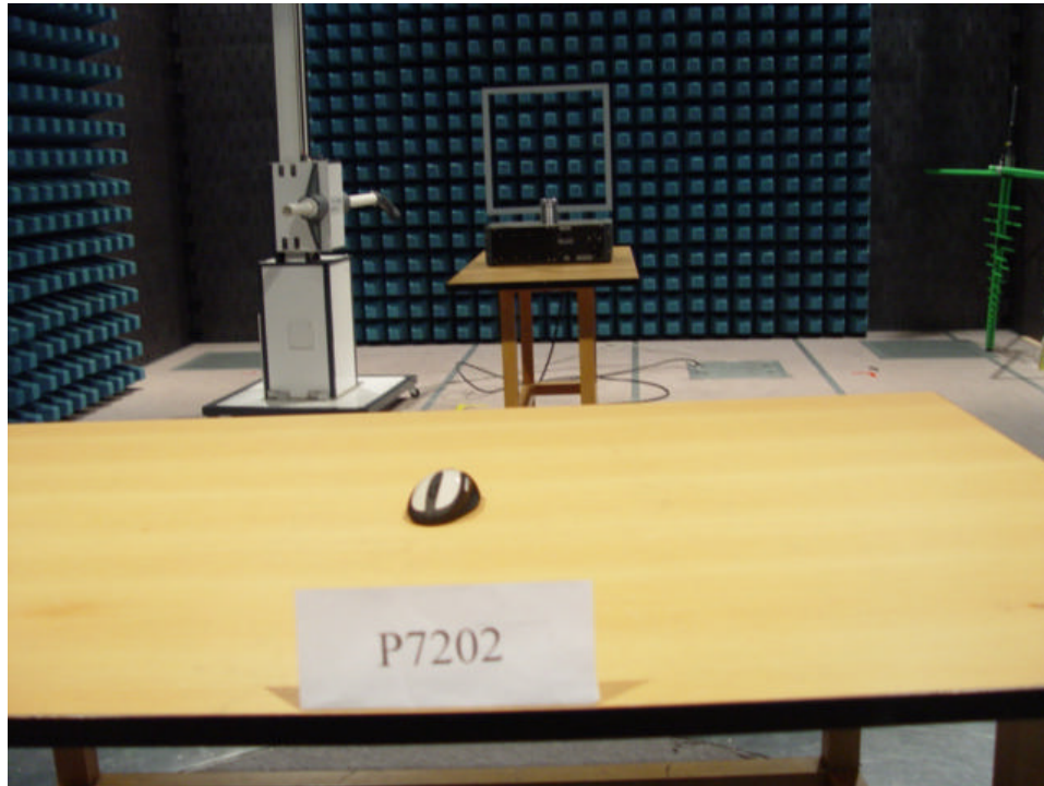
Photograph 1: Set-up for Radiation Measurement Below 30MHz
