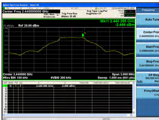
GFSK MIDDLE CHANNEL, CARRIER LEVEL
