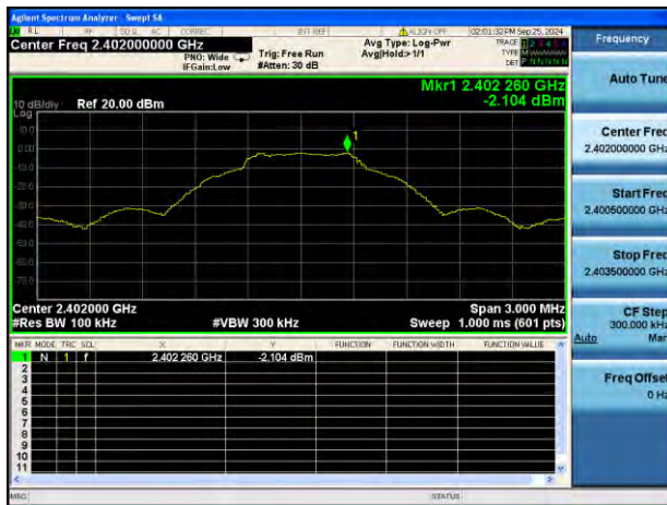
GFSK LOW CHANNEL, CARRIER LEVEL
