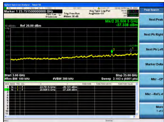
GFSK LOW CHANNEL, SPURIOUS 3 GHz ~ 25 GHz
