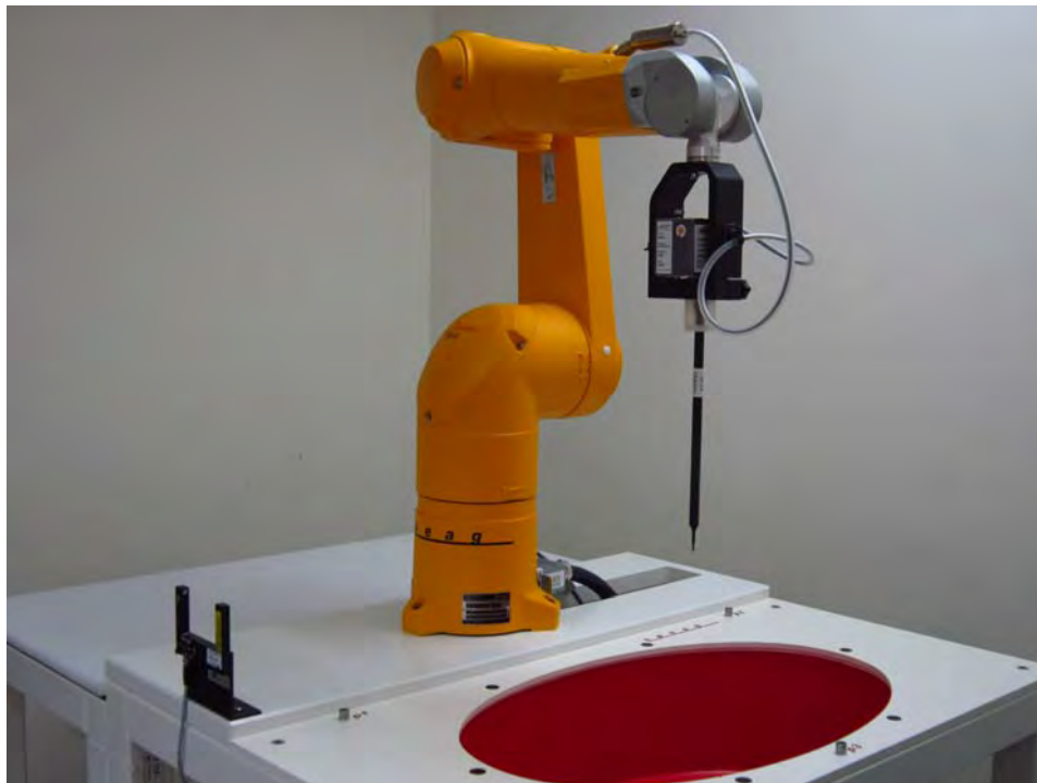
Fig.1 Photograph of the SAR measurement system
