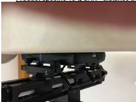
Fig.9 EUT Front side to flat phantom
