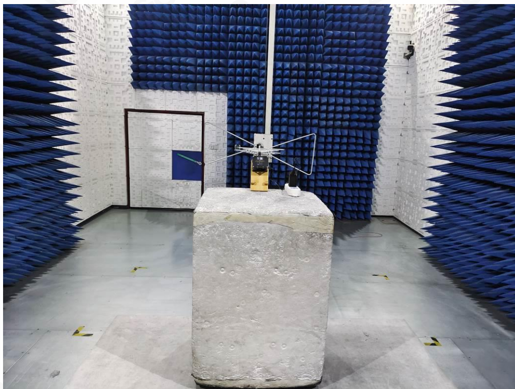
FCC RADIATED EMISSION TEST SETUP 30MHz-1GHZ
