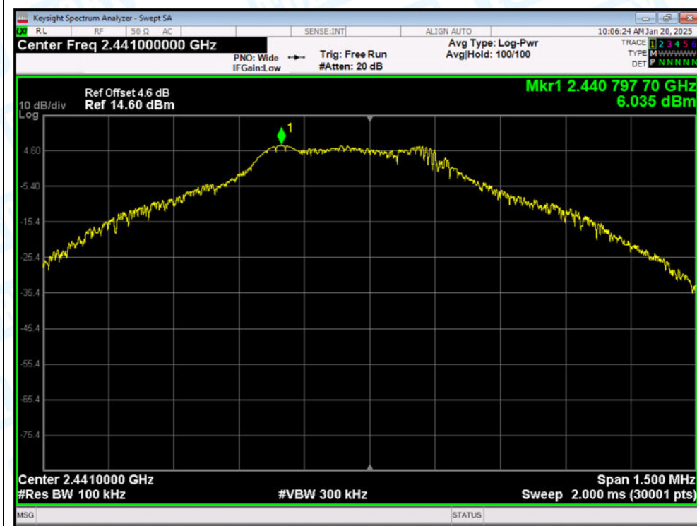
Tx. Spurious NVNT 1-DH1 2441MHz Ant1 Emission
