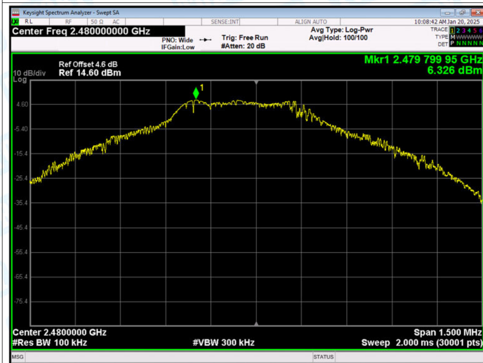
Tx. Spurious NVNT 1-DH1 2480MHz Ant1 Emission
