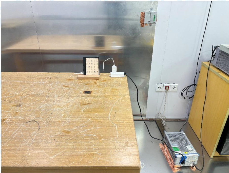
Photo of Setup for Conducted Emission
