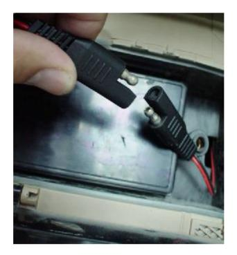
• Remove the battery connector from the M1A2 Abrams Tank harness connector.
