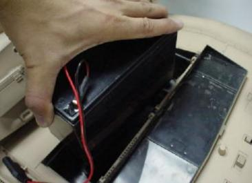
• ATTENTION: Make sure the battery connector wires connected to the same color of the battery pole i.e. black color wire connector connected to black color battery pole (-ve) and red color wire connector connected to red color battery pole (+ve).Place the 12 Volt (7.0 Amp/Hr.) battery upright in the battery compartment. Make sure the battery
