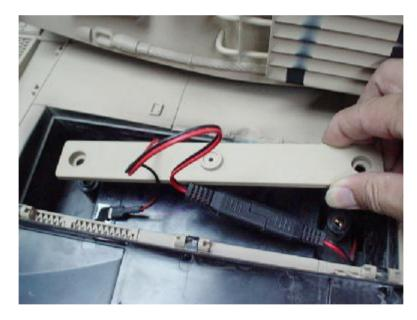
• Position the battery clamp over the battery with the ends of the battery clamp aligned with the screw holes in the battery compartment.
