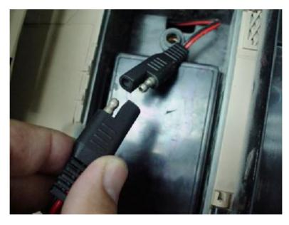
• Plug the battery connector into the M1A2 Abrams Tank harness connector.
