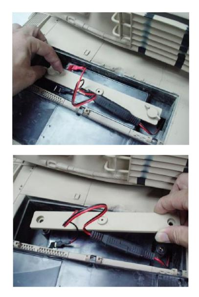
• Loosen the butterfly screws from the battery clamp. Remove the battery clamp from the battery compartment.
