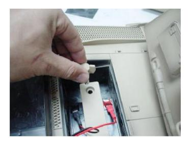
• Insert the butterfly screws through the ends of the battery clamp into the battery compartment.
