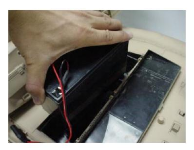
• Remove the 12 Volt (7.0 Amp/Hr.) battery from the battery compartment.
