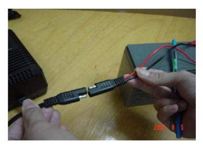
• Plug the charger connector into the battery connector.
