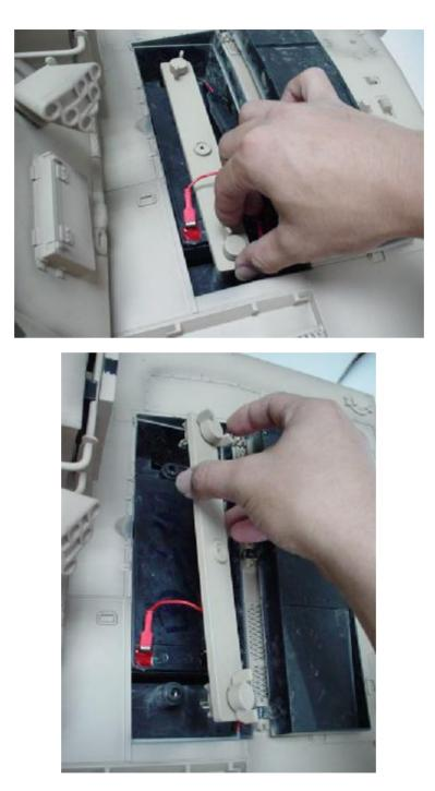
• Loosen the butterfly screws from the battery clamp. Remove the battery clamp from the battery compartment.
