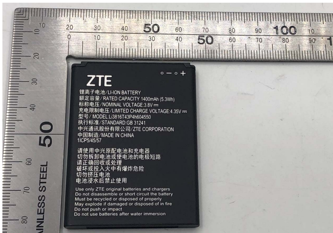
The battery front view (Li3816T43P4h604550 made by NINGBO Veken Battery.)
