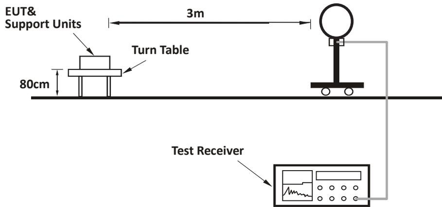
For Radiated emission 30MHz to 1GHz:
