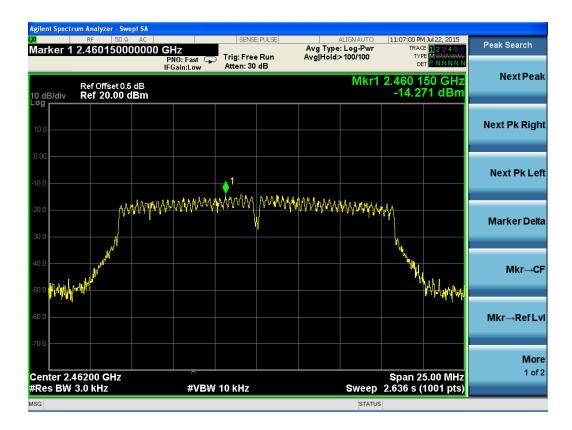
This report shall not be reproduced except in full, without the written approval of Shenzhen LCS Compliance Testing Laboratory Ltd.. Page 18 of 59 802.11n HT20 power density
