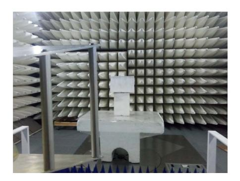
Photograph No.4 Setup for spurious emission field strength measurements in the anechoic chamber, EUT close view
