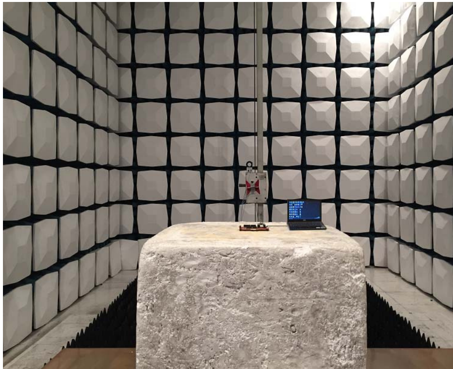
Description: Radiated Emission Test Setup for 1~18GHz
