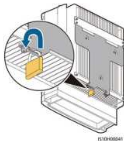
Figure 4-6 Opening the anti-theft lock
