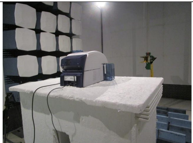
Radiated Emissions (>1GHz) – Rear View
