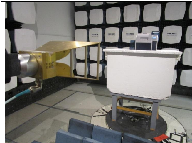
Radiated Emissions (>1GHz) – Front View
