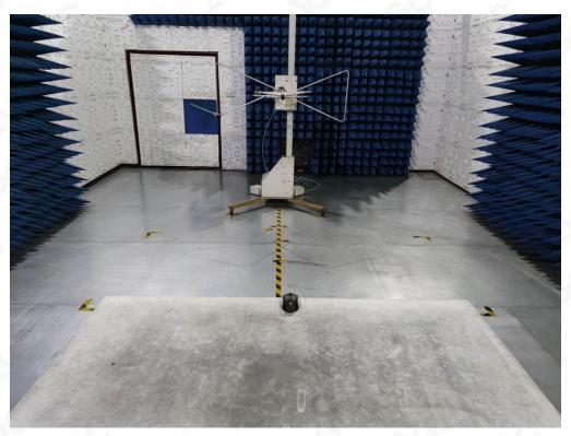
RADIATED EMISSION TEST SETUP ABOVE 1GHz
