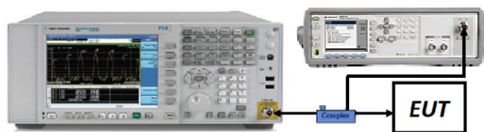
Figure 7-5. Test Instrument & Measurement Setup
