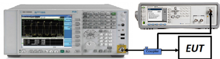
Figure 7-6. Test Instrument & Measurement Setup
