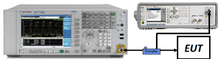
Figure 7-2. Test Instrument & Measurement Setup
