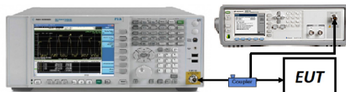
Figure 7-3. Test Instrument & Measurement Setup
