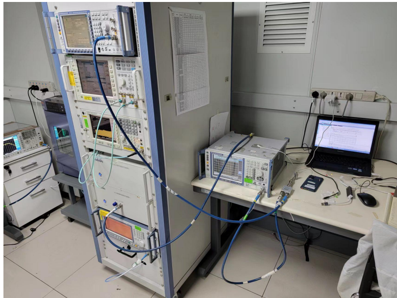
RF Conducted Test setup (GSM/WCDMA/LTE)
