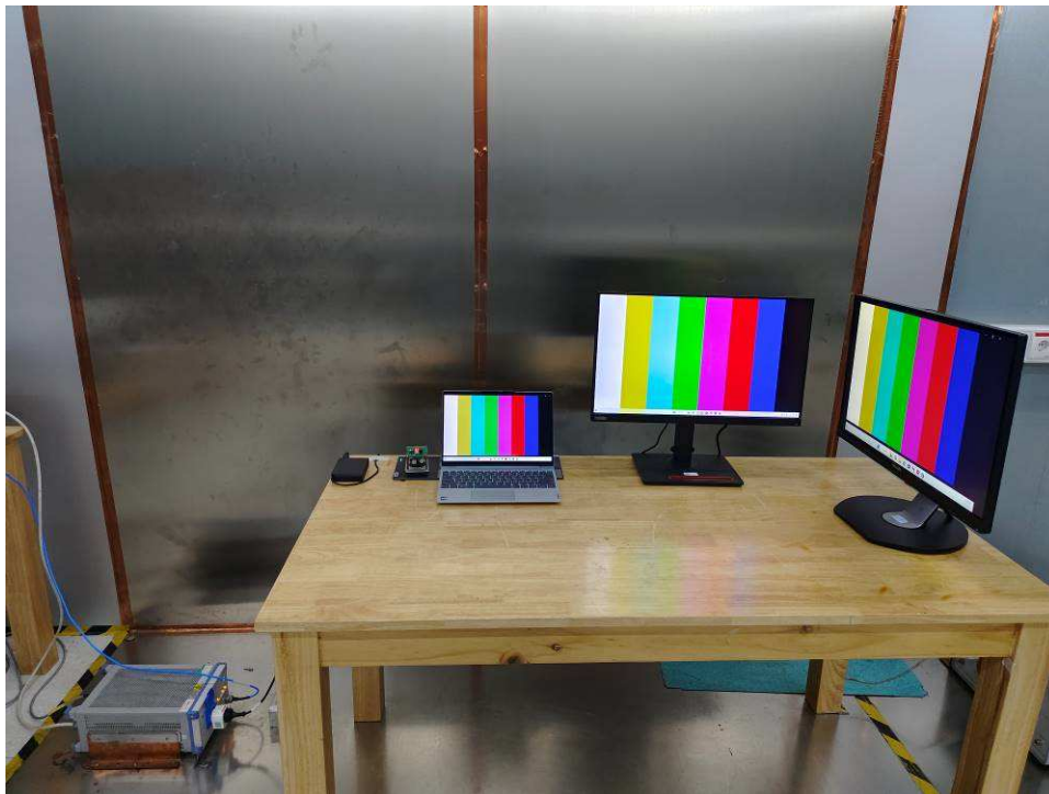
Photograph 1: Set-up for Conducted Emission on AC Mains
