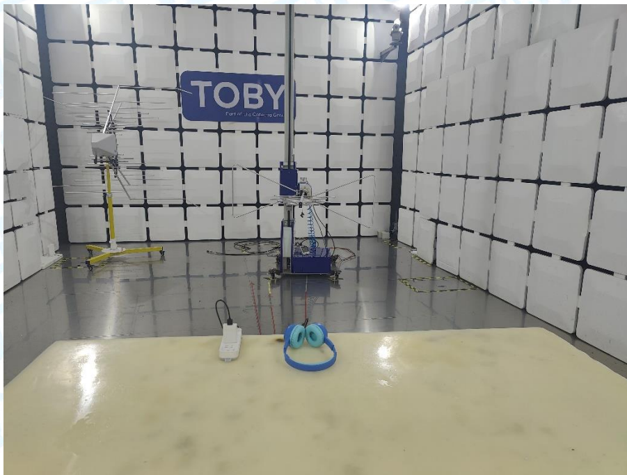
Photo of Setup for Radiated Emission (30MHz~1GHz)
