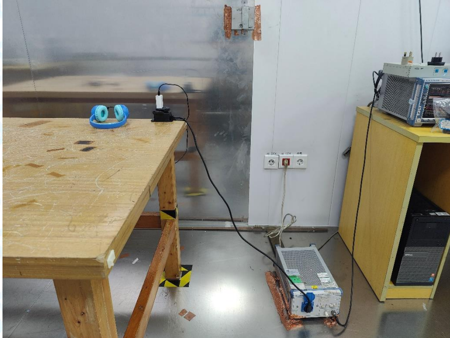
Photo of Setup for Radiated Emission (30MHz~1GHz)
