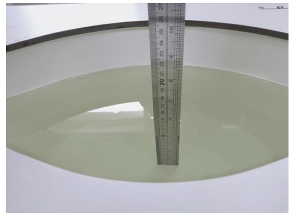
Liquid depth in the body phantom (2450MHz)
