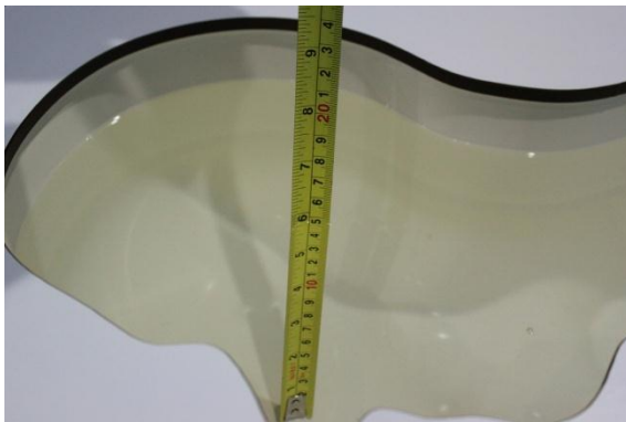
Liquid depth in the head phantom (1900MHz)
