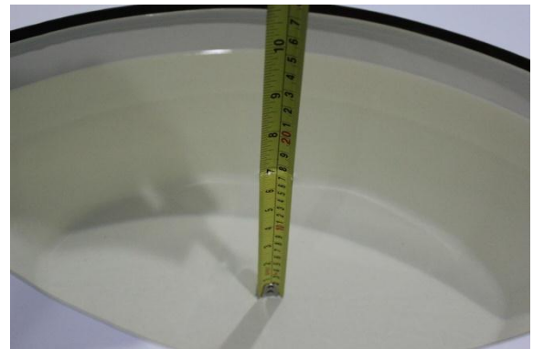
Liquid depth in the body phantom (1900MHz)
