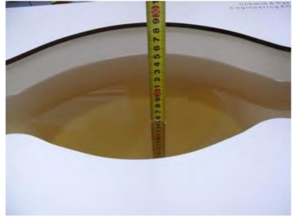
Liquid depth in the body phantom (835MHz)
