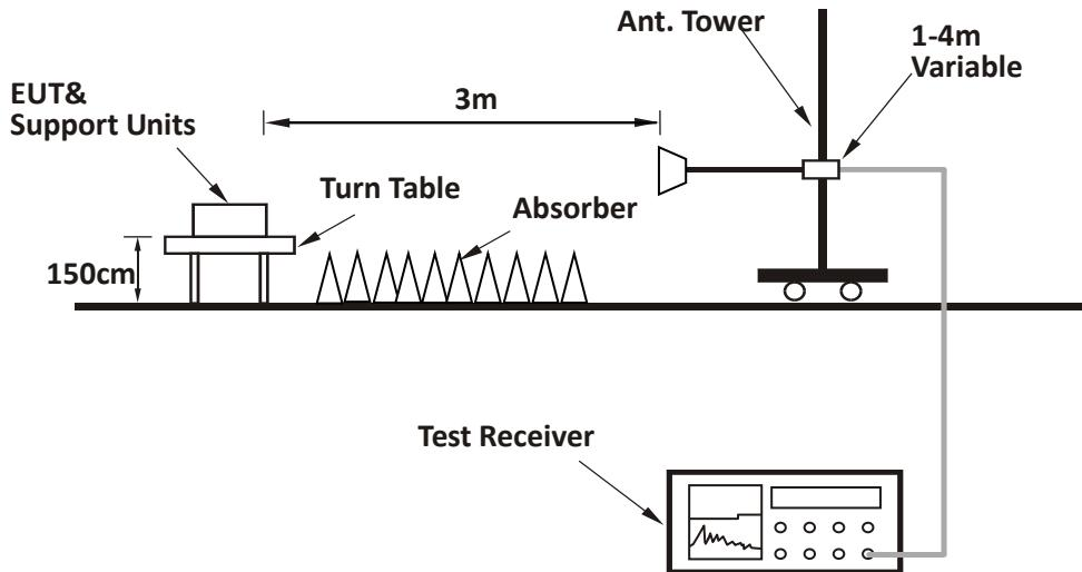
**TEST REPORT****7.4 Test Results of Radiated Emissions**
