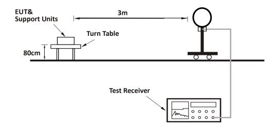
For Radiated emission 30MHz to 1GHz:
