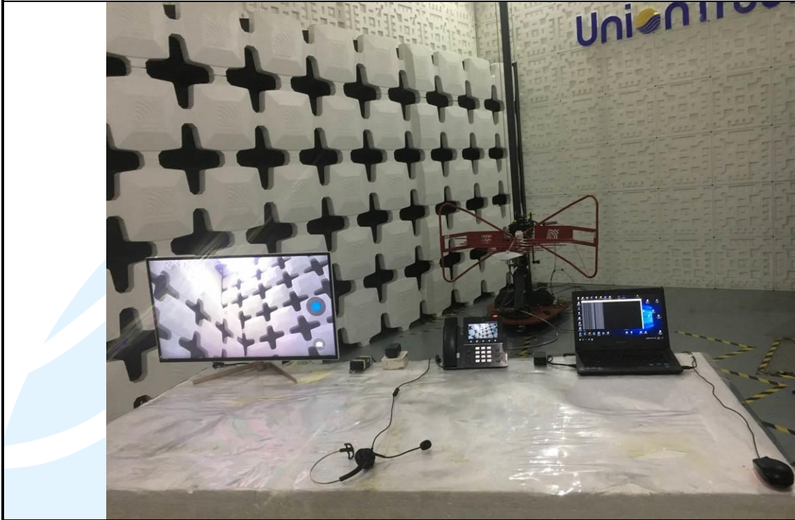
Radiated emission Test Setup-1 (30 MHz~1 GHz) _Test Mode 4
