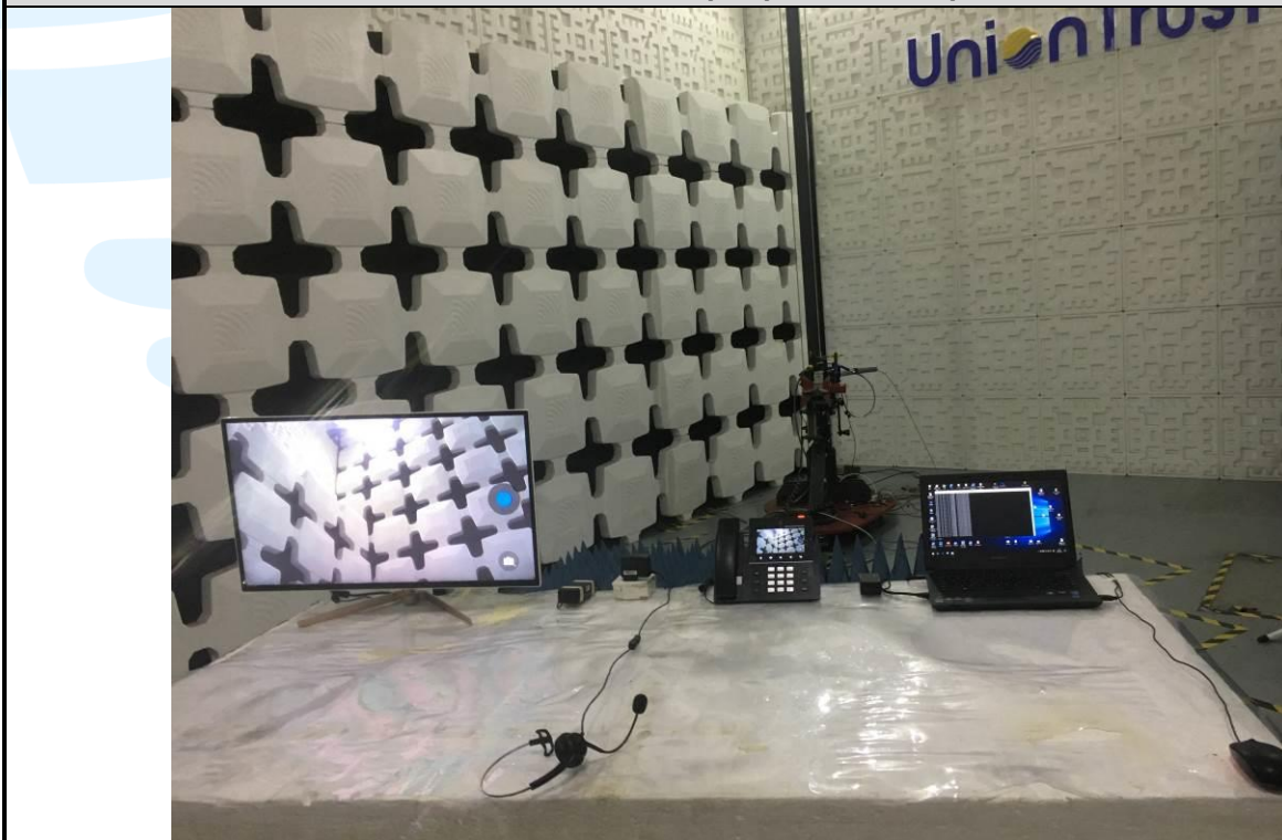
Radiated emission Test Setup-2 (Above 1 GHz) _Test Mode 6
