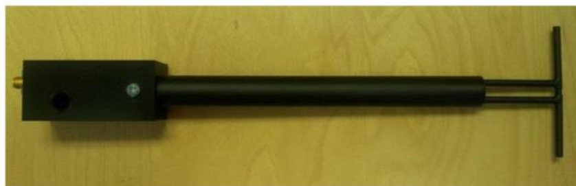
Figure 1 – MVG COMOSAR Validation Dipole
