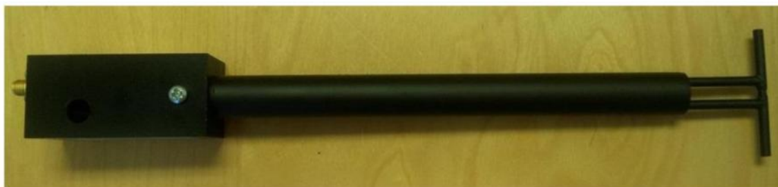
Figure 1 – MVG COMOSAR Validation Dipole
