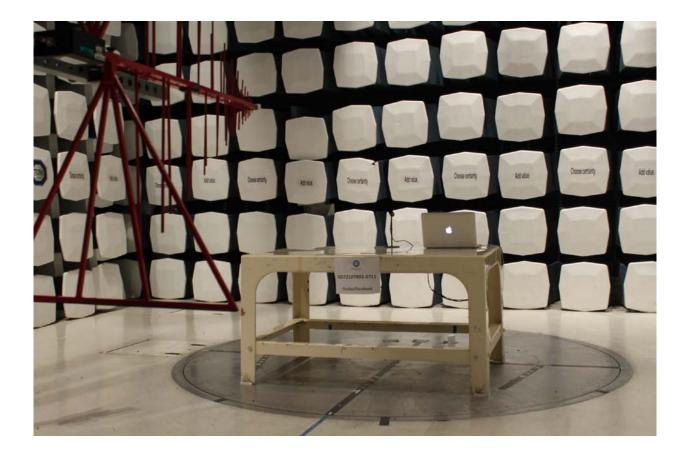
Radiated Emissions Test Setup (below 1GHz)
