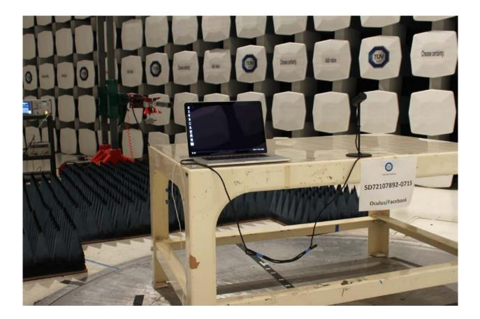
Radiated Emissions Test Setup (above 1GHz)
