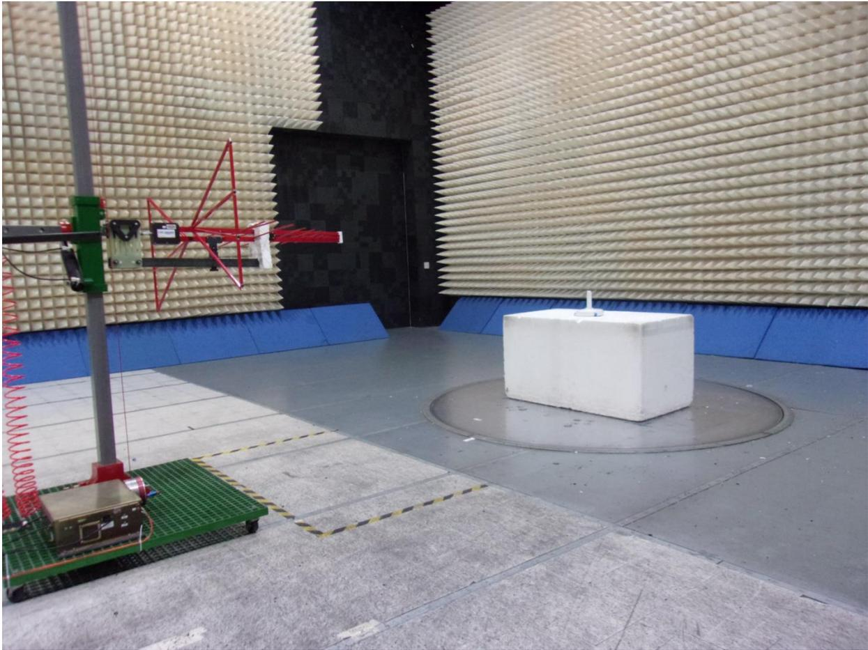
Figure 2 – Radiated Spurious Emissions, 30MHz – 1GHz
