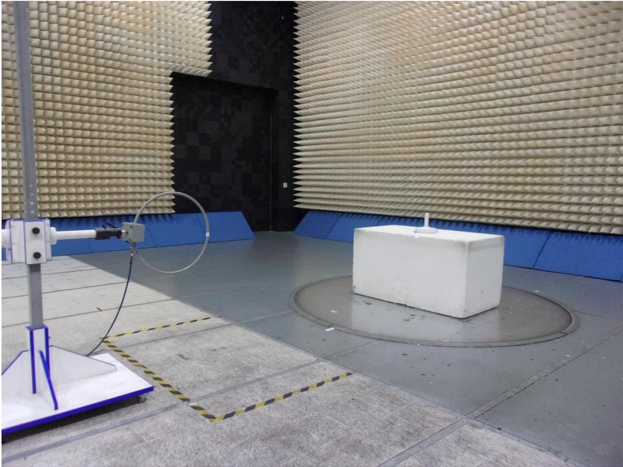
*Figure 3 – Radiated Spurious Emissions, 9kHz – 30MHz*
