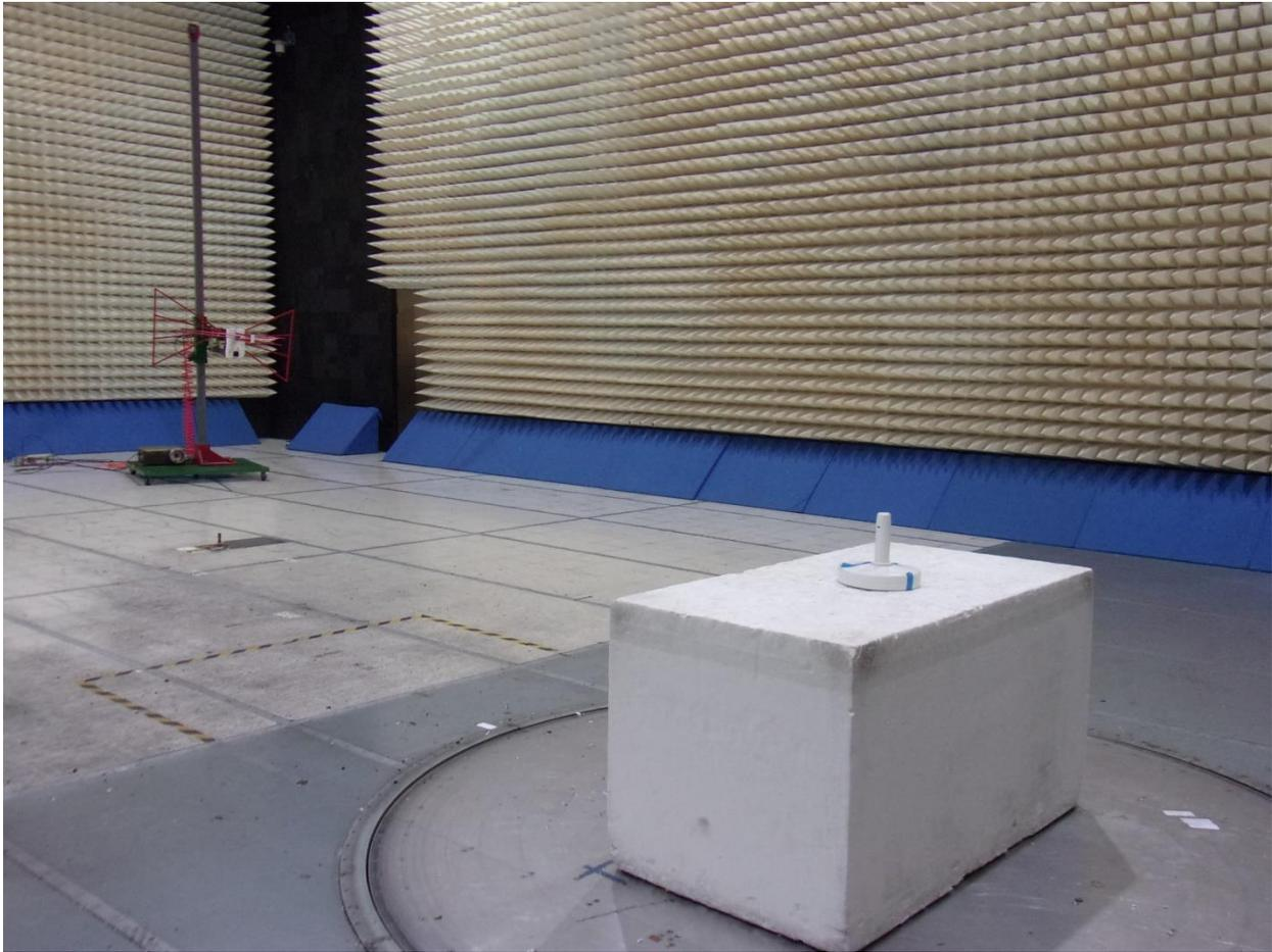
*Figure 1 – Unintentional radiated Emissions, 30MHz – 1GHz*
