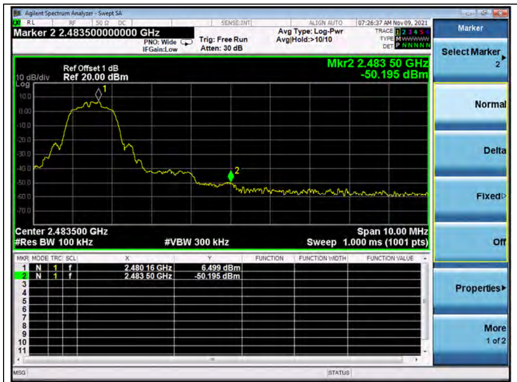
(Band edge, Channel 78, \pi/4 -DQPSK)
