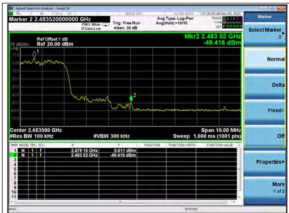
(Band edge with hopping on, Channel 78, 8-DPSK)
