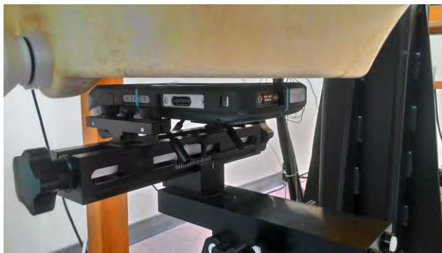
Fig.3 EUT front side to flat phantom
