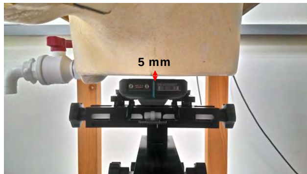
Fig.3 EUT front side to flat phantom
