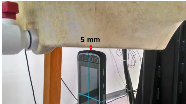
Fig.7 EUT bottom side to flat phantom
