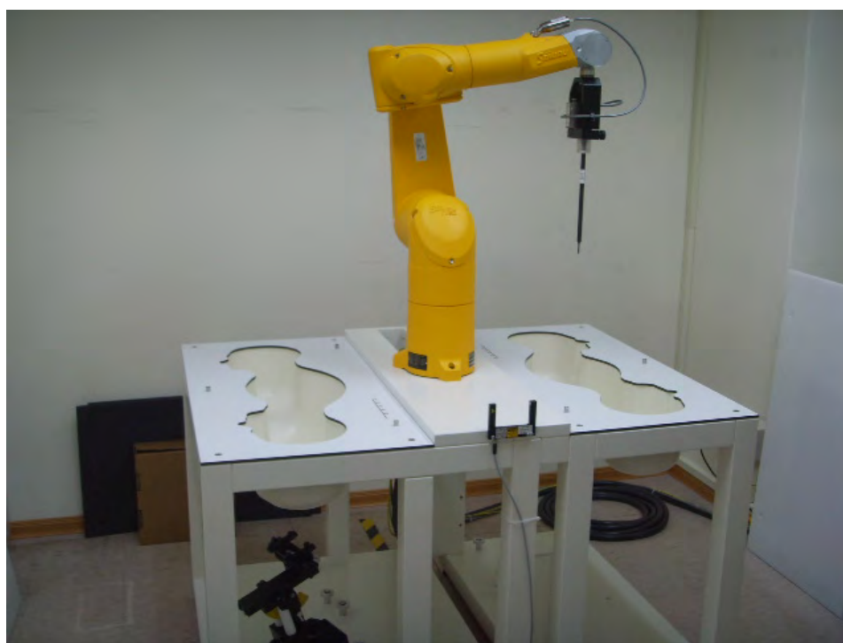
Fig.1 Photograph of the SAR measurement system
