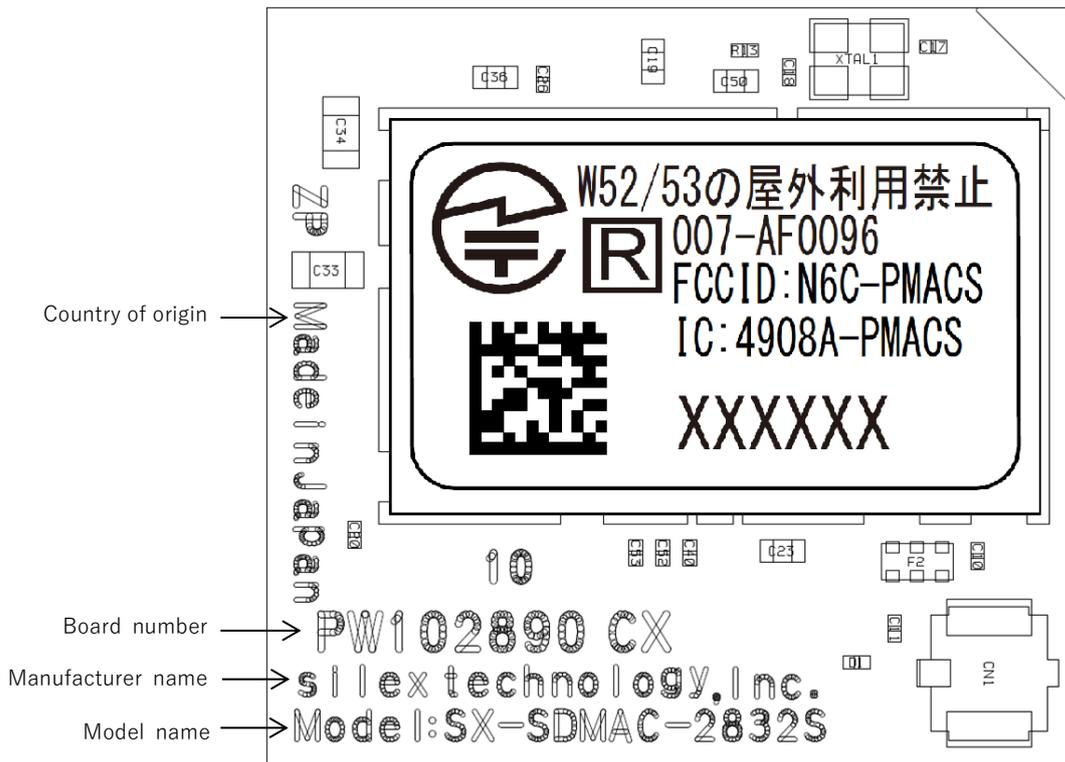
The Label is placed on the RF shielding case.
