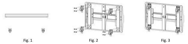
2. Connect the base screws to the product base and the product body, and tighten all the base screws with an Allen wrench.
