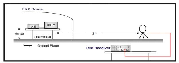
Below 1GHz Test Setup:
