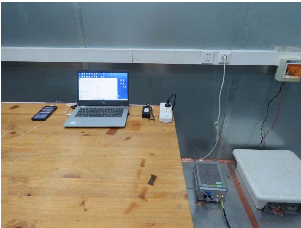
Picture 1: Conducted Emissions Test Setup
