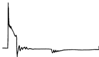
Secondary circuit resistance is too large
