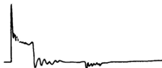
Oil or coke was attached in spark plug
