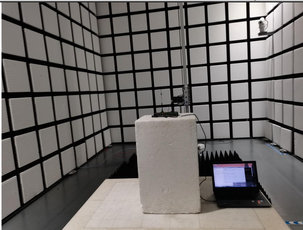
Radiated emission setup photo(Above 1GHz)
