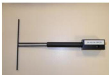
Figure 1 – Satimo COMOSAR Validation Dipole
