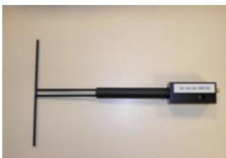
Figure 1 – Satimo COMOSAR Validation Dipole
