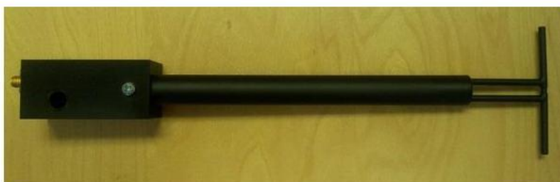
Figure 1 – MVG COMOSAR Validation Dipole
