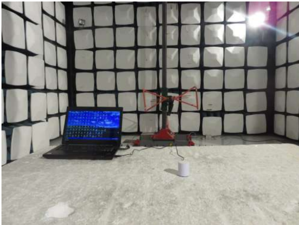
FCC RADIATED EMISSION TEST SETUP
