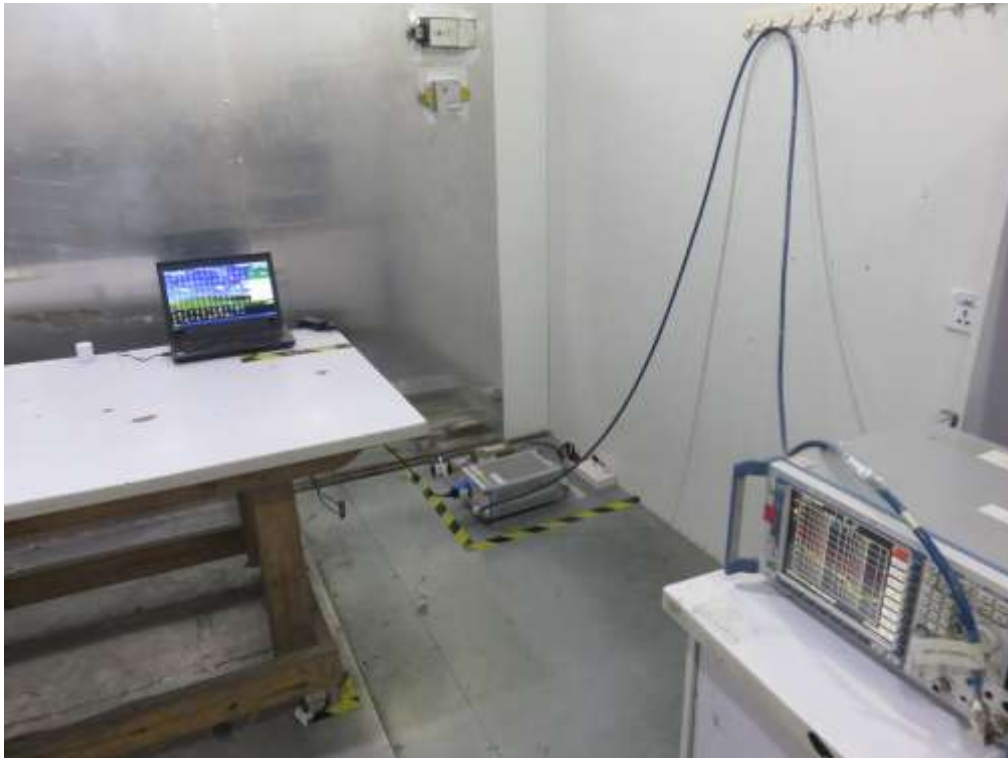
FCC RADIATED EMISSION TEST SETUP
