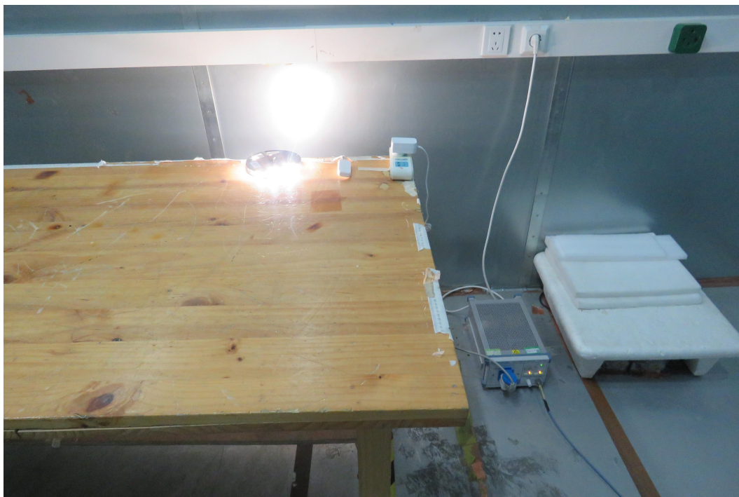
Picture 3 Conducted Emission Test Setup
