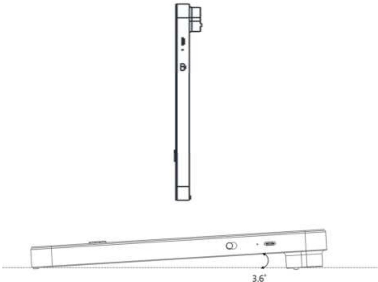
On the right side of the Dot Pad 320, starting from the rear to the front, there is a USB C type power charging port, followed by a power switch. A USB C type power port is a power only port. Keep in mind that there is no data transfer.
