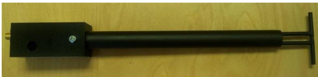
Figure 1 – MVG COMOSAR Validation Dipole
