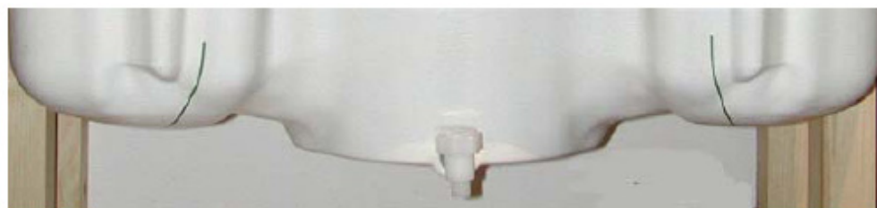
Figure 7.2 SAM Twin Phantom shell
