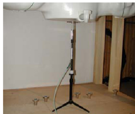
Figure 12.1 Dipole Validation Test Setup
