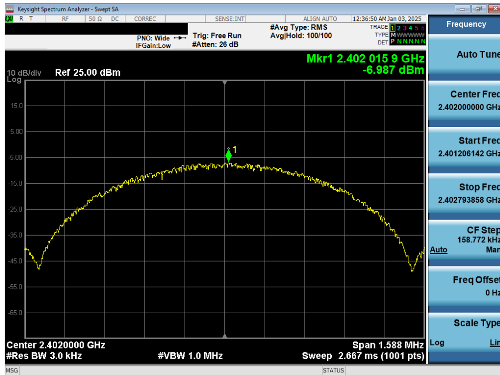
Plot 7-28. Power Spectral Density Plot Antenna WF7b (Bluetooth (LE), 1Mbps, iPA – Ch. 0)
