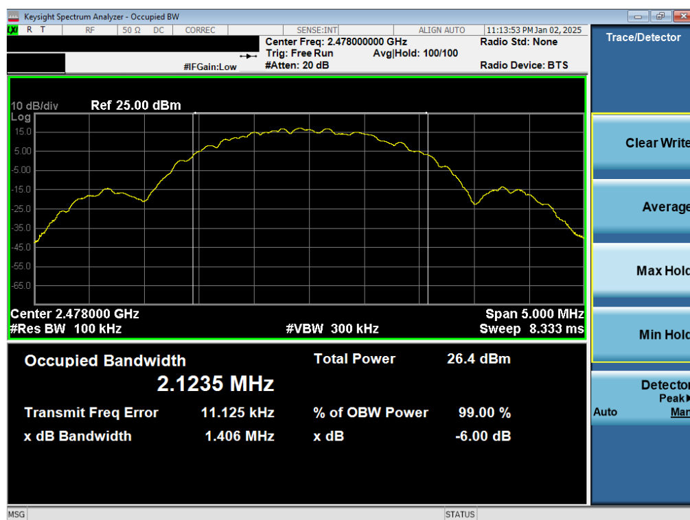
Plot 7-6. 6dB BW & 99% OBW Plot Antenna WF8 (Bluetooth (LE), 2Mbps, ePA – Ch. 38)
