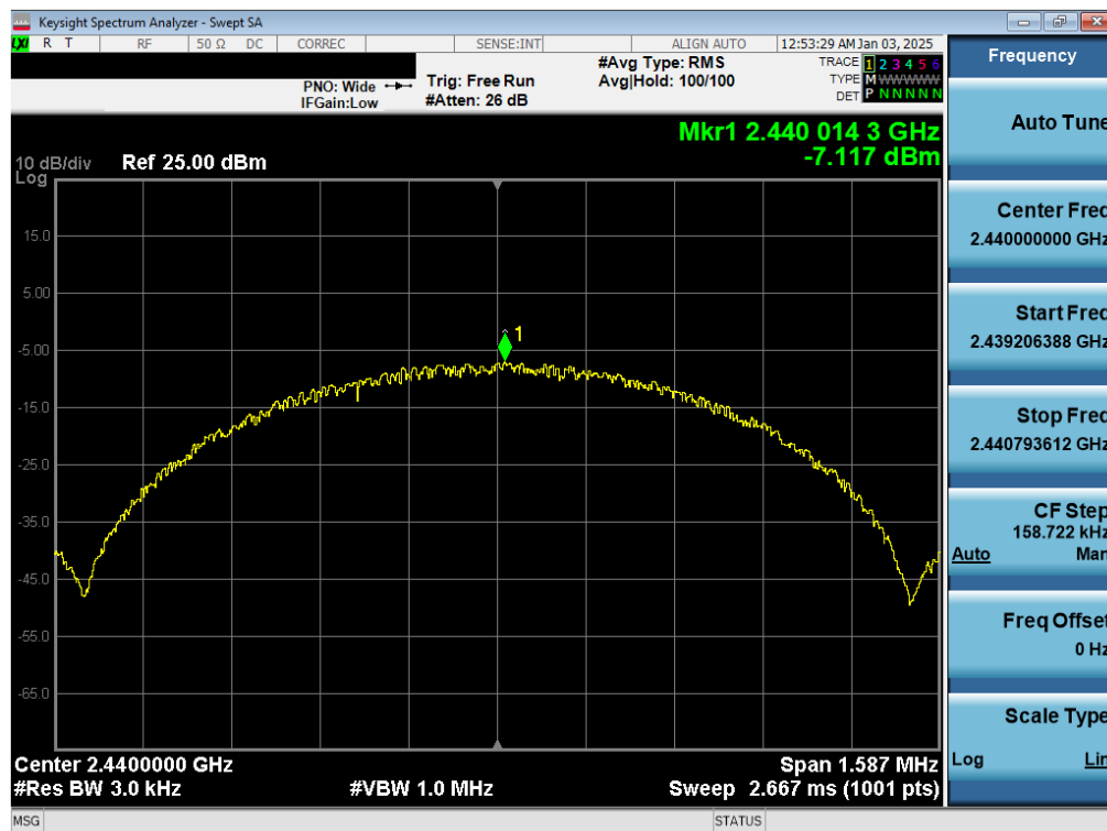
Plot 7-46. Power Spectral Density Plot Antenna WF7b (Bluetooth (LE), 1Mbps, iPA – Ch. 19)
