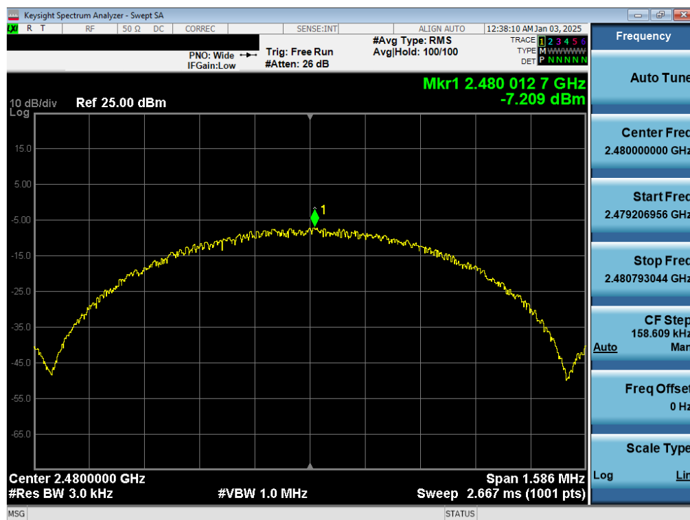
Plot 7-30. Power Spectral Density Plot Antenna WF7b (Bluetooth (LE), 1Mbps, iPA – Ch. 39)
