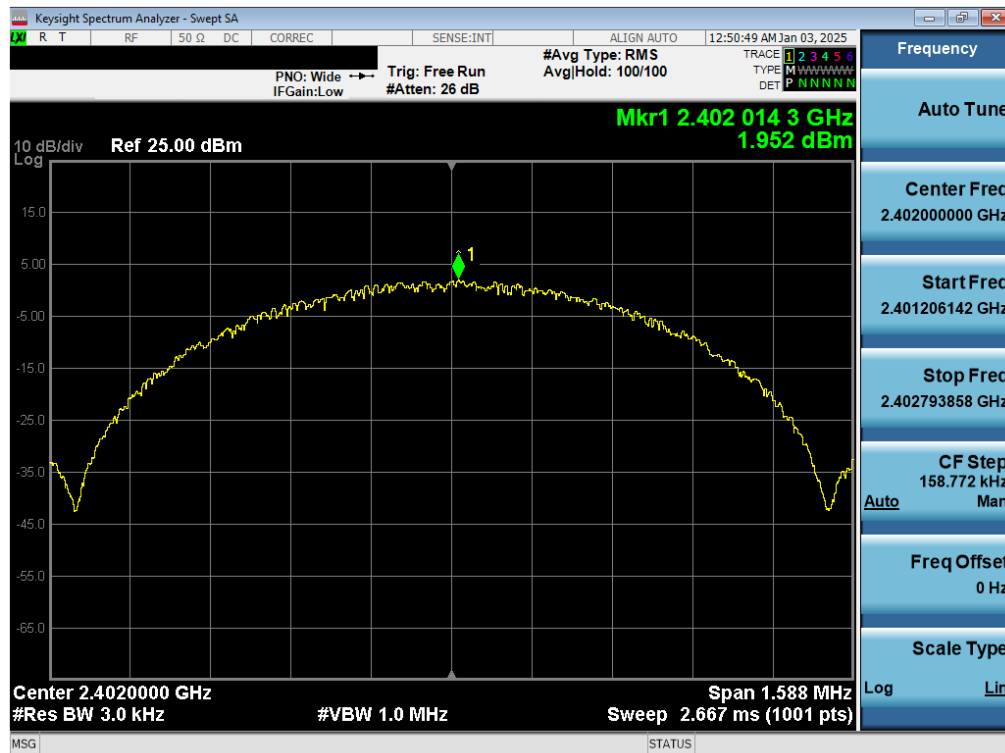
Plot 7-38. Power Spectral Density Plot Antenna WF7b (Bluetooth (LE), 1Mbps, ePA – Ch. 0)
