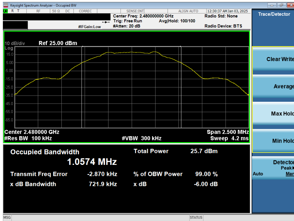
Plot 7-9. 6dB BW & 99% OBW Plot Antenna WF7b (Bluetooth (LE), 1Mbps, ePA – Ch. 39)
